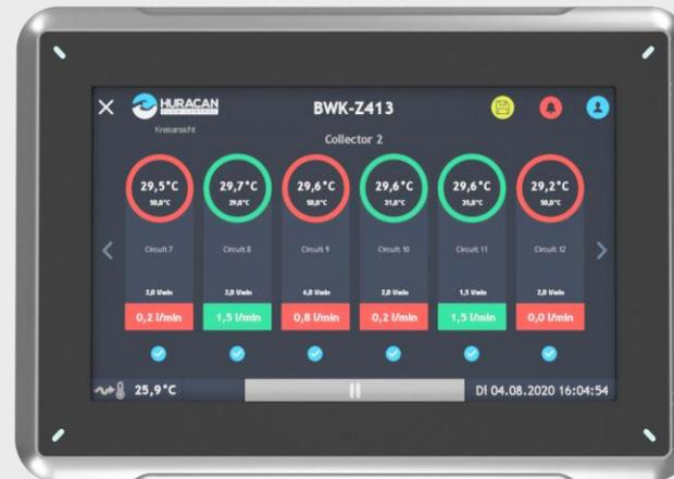
Define the upper and lower limits and set the target values for each circuit.
